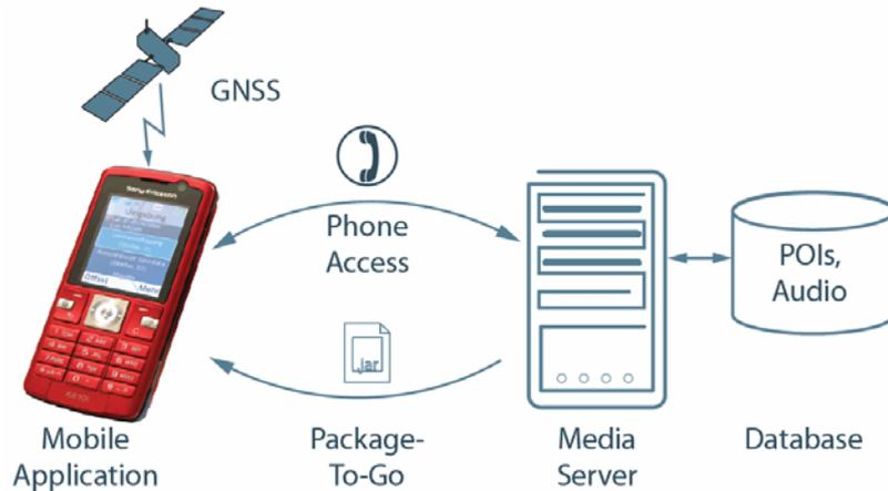
Figure 3. Architecture and concept of the MontaPhone communication
