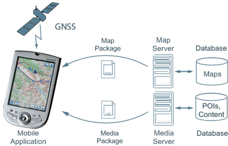
Figure 5. Communication and deployment architecture of the SmartGuide
